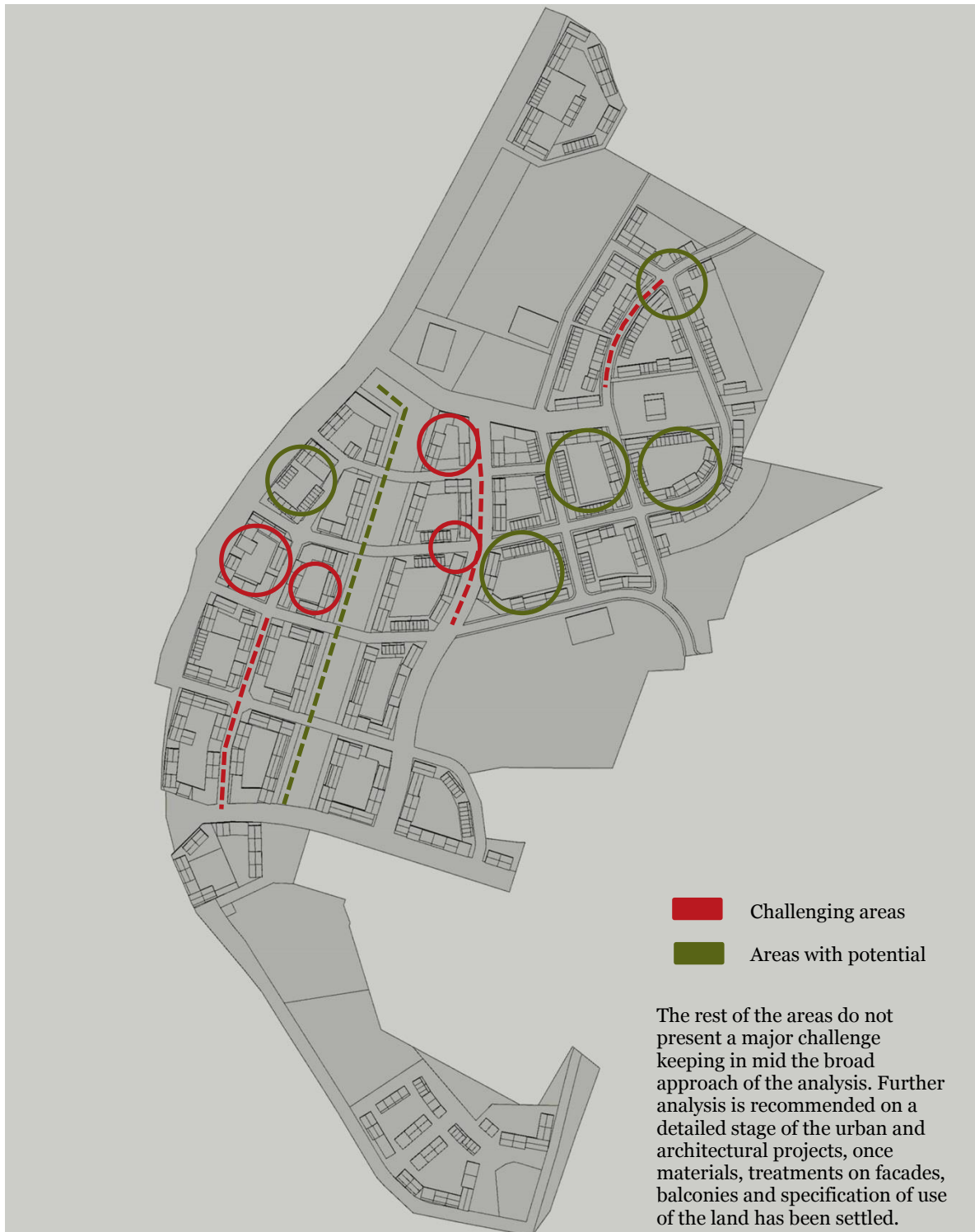
Figure 15 : Identification of areas with potential and challenging areas in relation to Available Daylight Provision on the facades and Window-to-Wall Ratio performance
